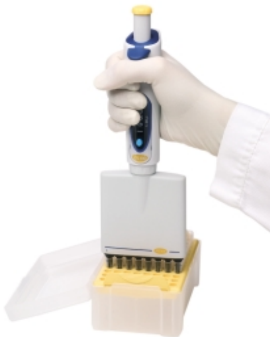
Figure 3 The Optiload system features spring-loaded tip cones that allow pipettor tips to be picked up with a constant force. This, in turn, ensures even tip sealing and sample pickup, and considerably reduces tip ejection force compared to conventional pipettors.
